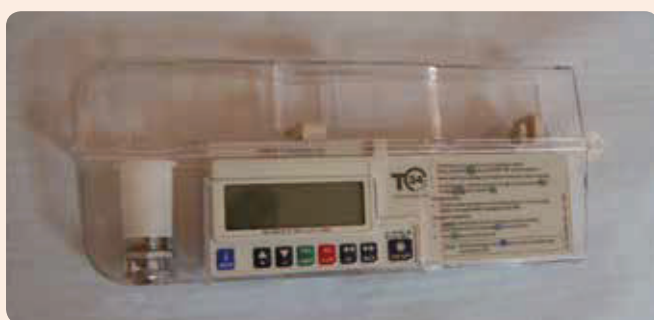
Fig. 4 Syringe pump mechanism for continuous medications (no syringe attached)
